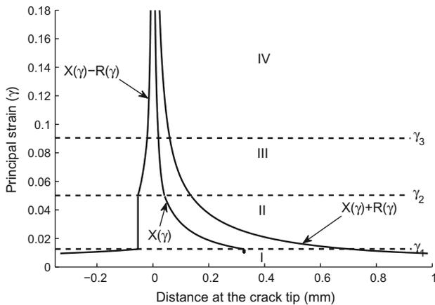
Fig. 8. Evolution of  $X(\gamma)$  and  $R(\gamma)$  of the circle of constant strain along the X-axis.
