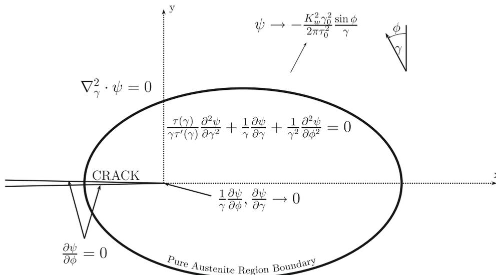
Fig. 1. Formulation of the edge crack problem for a material subjected to antiplane strain.
