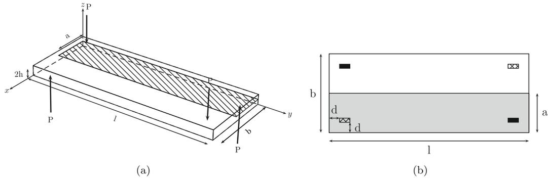
**Fig. 4.** (a) A top view of the Nickel–Titanium specimen used in the finite element analysis. The hatched zone in (a) represents the cracked region of the sample. (b) The zones where a uniform pressure is applied. On the upper face these zones are shown in black, hatched on the lower face. The area of one zone is equal to 1.14 mm<sup>2</sup>.
