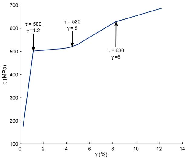
**Fig. 5.** stress–strain relation between  $\gamma$  and  $\tau$  obtained in the simulation.
