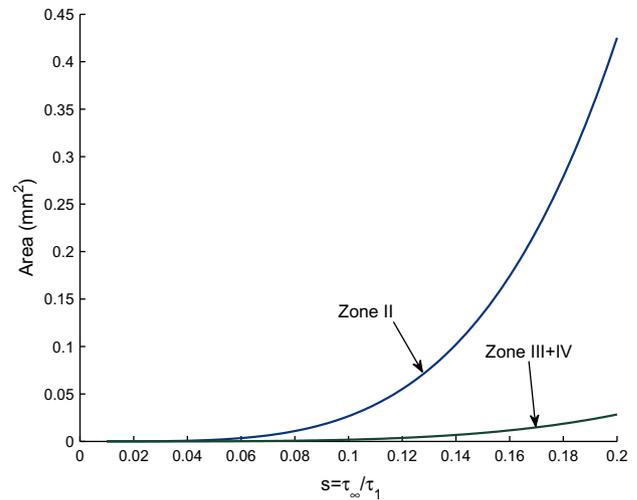
Fig. 9. Evolution of the area of the Zones II–IV with the remote applied stress.
