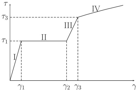
Fig. 2. Model for the mechanical behavior of a shape memory alloy.
