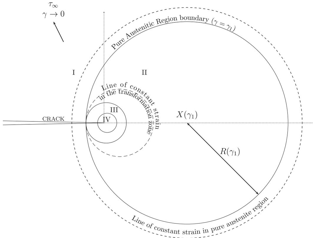
**Fig. 3.** Geometry of small-scale yielding near a crack for a model of SMA under mode III loading.
