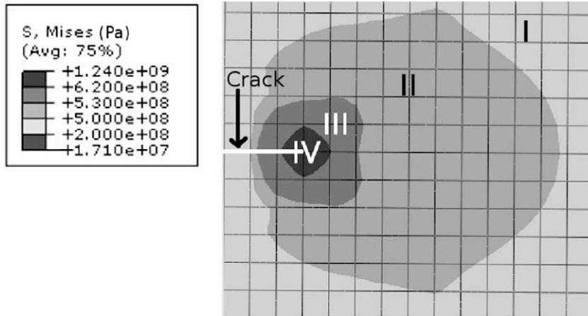
Fig. 7. Mises stress ( $\tau$ ) in Pa around the crack tip for  $y=45$  mm. Applied pressure : 5.5 GPa,  $s = 0.19$ .
